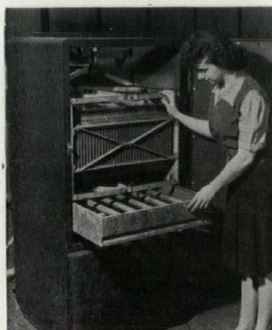
Right, Westinghouse "Precipitron," cabinet type for houses, collects dust from the atmosphere
