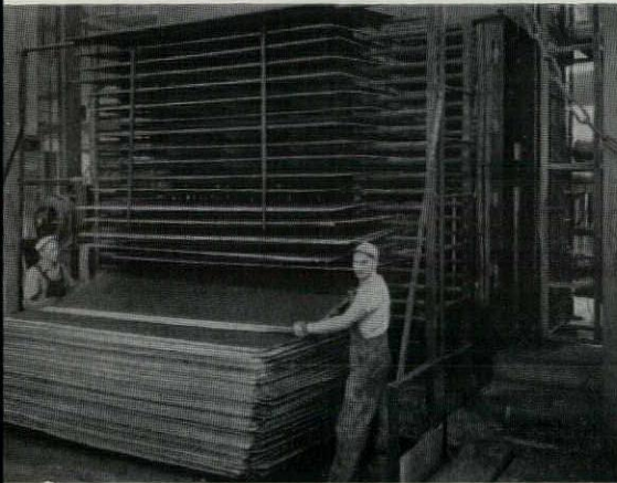
Above, left, manufacturing plastic-surfaced plywood; right, manufacturing part of a plane wing of wood plies, indicating the many structural possibilities of formed plywood
