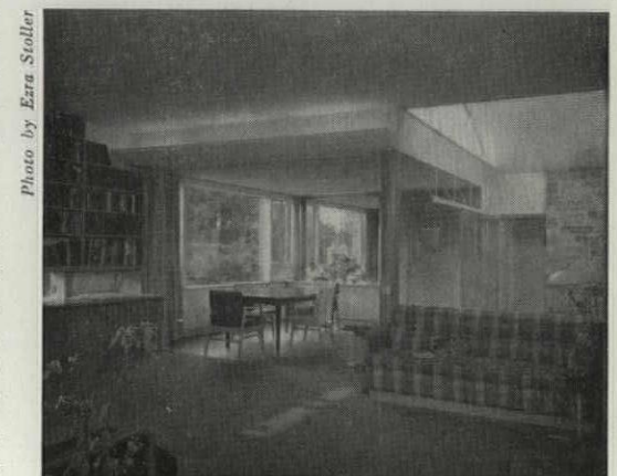
Fluorescent ceiling trough provides general lighting in the living room of the same house shown above. Local lighting is provided by incandescent portable and fixed lights.
