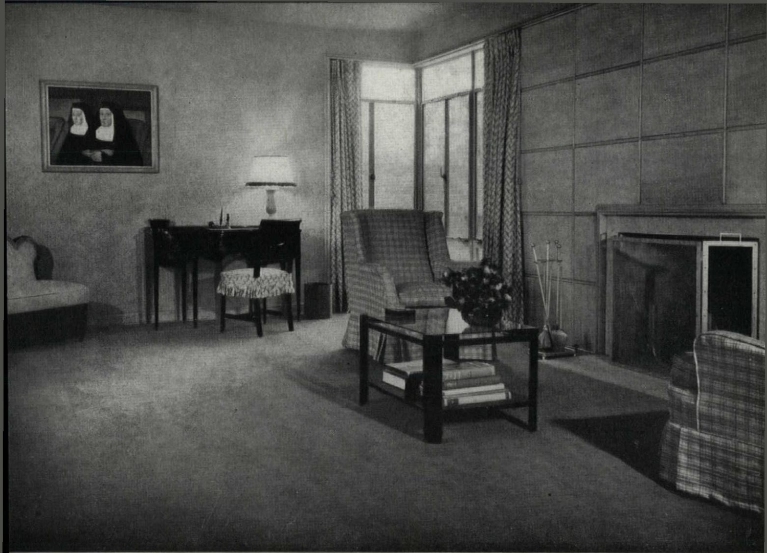
Fireplace wall of living room paneled in plywood
