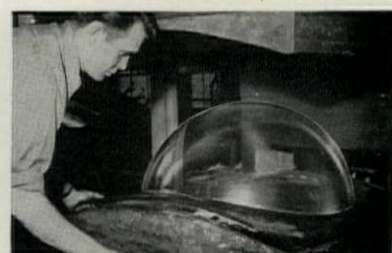
FABRICATED ACRYLICS: LEFT, Plexiglas cabinet shelves, transparent, shatterproof; rounded, easily cleaned corners. CENTER, surface-engraved Plexiglas. RIGHT, "bubble" shape formed by air pressure; material is a laminate of Lucite and another plastic; each imparts certain properties to the product.
