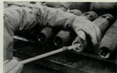
LIGHT CONTROL with acrylics: LEFT, new star-studded ceiling, Grand Central Station, New York City; CENTER, Lucite light conductors of different sizes used in the ceiling to transmit light from a single source to many stars. RIGHT, acrylic torch for inspecting interiors of shell parts.
