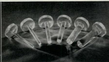
LIGHT CONTROL with acrylics: LEFT, new star-studded ceiling, Grand Central Station, New York City; CENTER, Lucite light conductors of different sizes used in the ceiling to transmit light from a single source to many stars. RIGHT, acrylic torch for inspecting interiors of shell parts.
