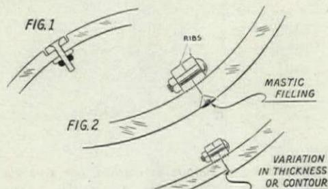
Multiple parts can be fastened together by mounting in a metal frame, as in Fig 1. This permits relatively thin panels. Fig. 2 shows another method, bolting together acrylic ribs cemented to circumferences of parts; matching formed parts may be difficult, outside contour of draw-formed pieces may vary; edges may be chamfered and joint filled.
