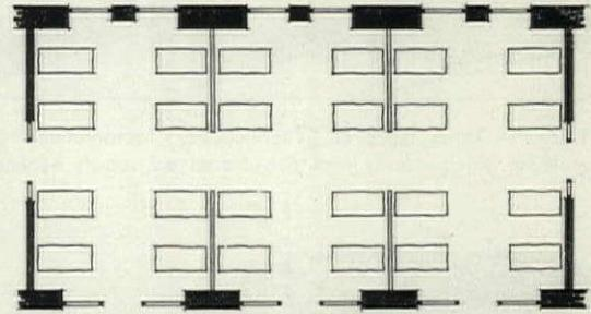
FIG. 16—Plan, typical 24-bed Riggs ward.
