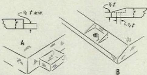
Cross section should be as uniform as possible, but assembly time may be saved by molding in mounting rims or lugs. These should be substantial; dimensions shown are minima, except that mounting holes are preferably of no greater diameter than  $\frac{1}{2} t$ , and should be set back from all edges of lugs a distance at least as great as thickness of the lug.
