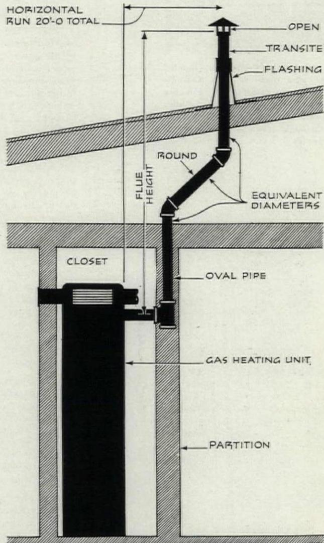
Diagram shows one method of installing new Type B flue approved for gas appliances only by Fire Underwriters. Made of asbestos-cement pipe, flue requires no masonry, can be supported on wood framing. According to A.S.H.V.E., total horizontal run should not exceed 20 ft in any case, and if flue height is less than 20 ft, horizontal run should not exceed flue height; other variables make competent advice necessary.
