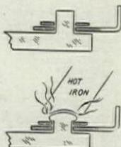
Molded acrylic "rivets," or short projecting lugs, can be used as shown for joining plastic and metal.
