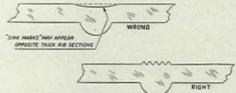
If ribs are used to reinforce an area, section may contract and shrink unevenly while cooling, due to greater volume of material. Cooling can be controlled to eliminate this but is expensive. Decoration of surface opposite rib overcomes the difficulty.
