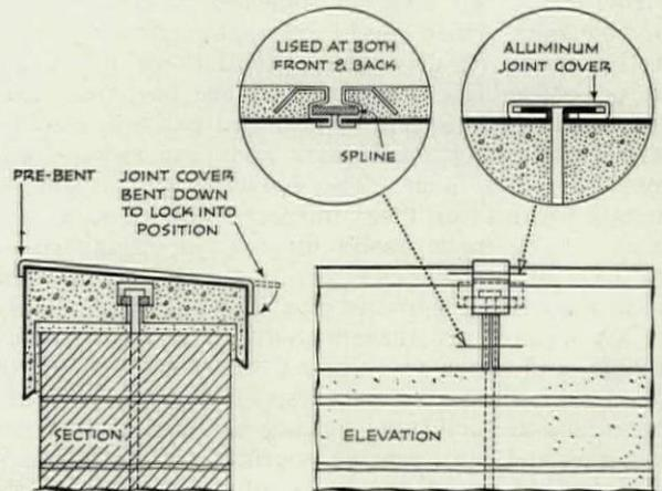
Method of capping a masonry coping—a detail necessary because many outmoded building codes still require masonry parapets.
