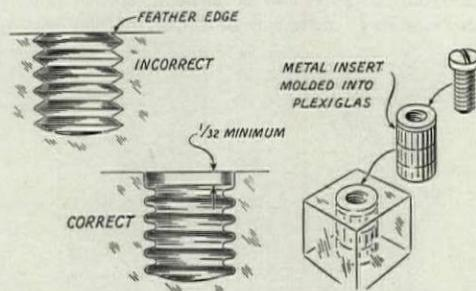
Screw threads may be molded rather than worked if hole diameter is  $\frac{1}{4}$ " or more; start threads at least  $\frac{1}{32}$ " down from surface, and avoid all sharp corners to avoid cracking. If part is to be disassembled often, metal inserts are preferable. Insert should be finished on outside because acrylics are transparent, should project slightly above surface of plastic. Proportions limited to depth not greater than twice diameter.
