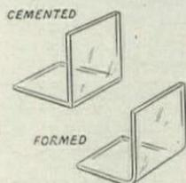
While cemented joints of good quality are easy to produce by handcraft methods, their quality is difficult to control in mass production. Particularly in decorative items, consider adding dye or pigment to cement rather than attempting completely transparent joints, or obscure joint with engraving or molding. Better still in many cases is a heat-formed joint.
