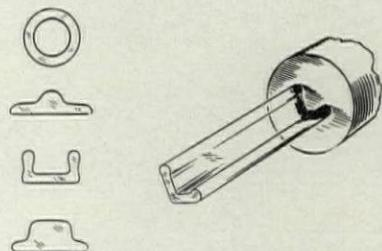
Many types of 3-dimensional moldings are possible, and advantage should be taken of the wide range of colors in which acrylics are available. For long parts in particular, extrusion is a fast, economical manufacturing method; it requires that the cross section or profile be uniform. Design should be discussed with an experienced extrusion molder.
