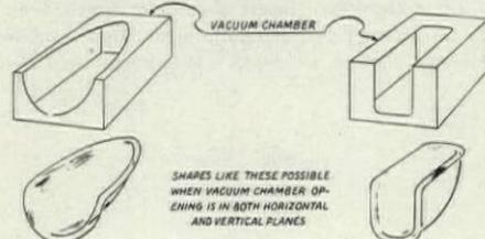
Types of vacuum-formed acrylic shapes and the forms (or "pots") which produce them. Called *surface tension shapes*, these have good optical properties. Material thins out, approximately 1/3 in a 22"-diameter hemisphere at deepest draw. In "snap-back" forming vacuum is reduced and material constricts to fit a male form of proper contour.
