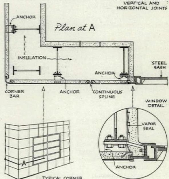
Details show essential elements of system. Method of assembly and further details appear on page 86.
