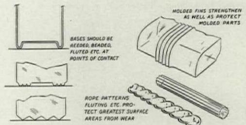
If roughly handled, surface of acrylics will be marred; hence, special surface treatments are desirable for parts likely to be scratched. They also break the surface into brilliant facets.
