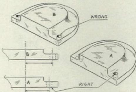
Keep mounting holes for panels or parts close to a thick portion of the panel; and if routing is to be done, keep width and depth of routing uniform to attain low production costs.
