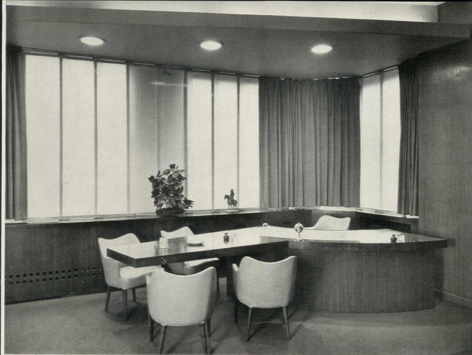
To shield the view, yet allow ventilation, top and bottom glass hinge louvers were installed over existing windows.
