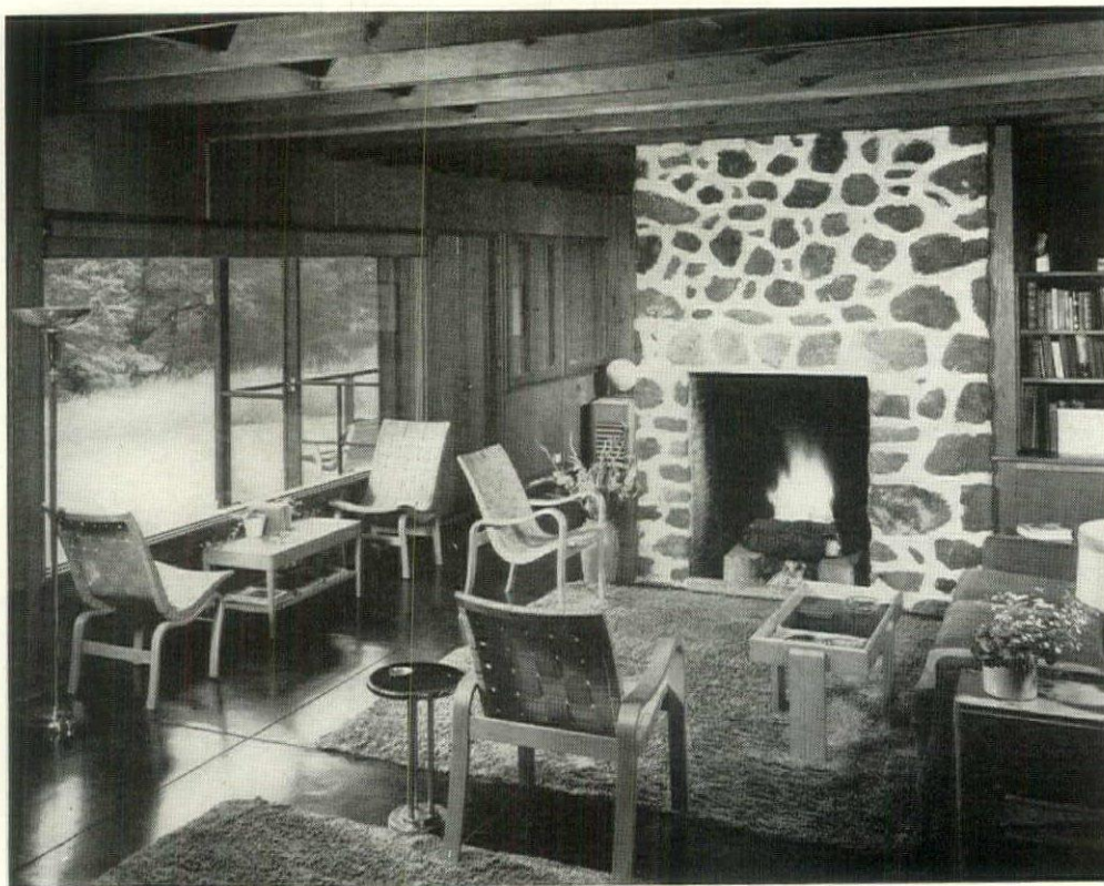
FIREPLACE. The fireback is of sheet steel that is top hinged from a channel-iron lintel in the center of the flue opening. The sheet may be swung from front to back and locked in either of two positions, thus serving two fireplaces—one, on the living-room side; the other, opening into the recreation room.
