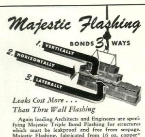
Majestic Flashing, fabricated from 16 oz. copper\* is the only corrosion and moisture proof material offering positive assurance against crumbling parapet walls due to seepage. Majestic Triple Bond Thru Wall Flashing is a sure, inexpensive safeguard against deterioration. Write today for the name of your nearest dealer and folder showing improved design. Nation wide distribution.
