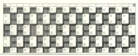
FRONT ELEVATION OF SIMPLEX ARRANGEMENT. As in the case of the three-story buildings, various patterns are made possible by reversing a typical two-bedroom apartment plan.
