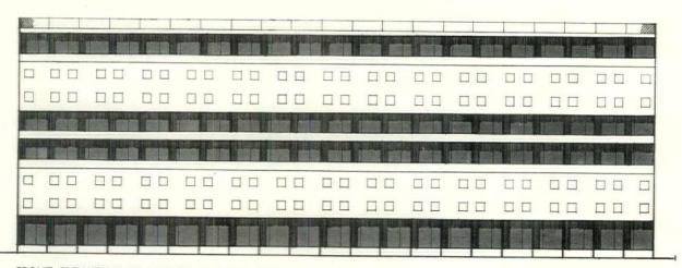
FRONT ELEVATION OF DUPLEX ARRANGEMENT. Pairs of bedroom floors are sandwiched between levels where duplex living rooms and the one-room apartments occur. Section shows the corridor and access to apartments at living-room floors.
