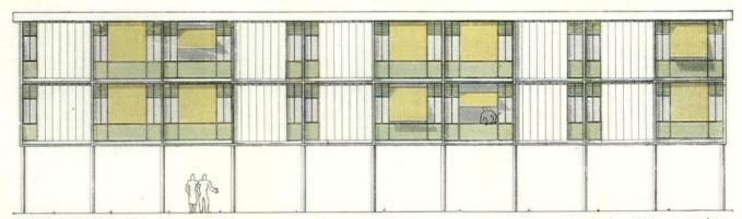
FRONT ELEVATION. Three of many facade patterns possible by alternating and reversing one typical apartment plan. Living rooms have louvred pivoting wall; bedrooms a single window on this elevation.
