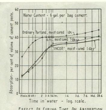
EFFECT OF CURING TIME ON ABSORPTION.
