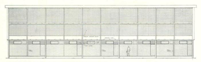
REAR ELEVATION. Outside corridors are protected by pierced masonry units.
