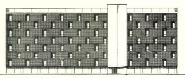
REAR ELEVATION OF SIMPLEX. The west facade of the simplex building presents seven floors of pierced-wall corridors above an open walkway. Occasional breaks in the corridor wall permit greater vision.
