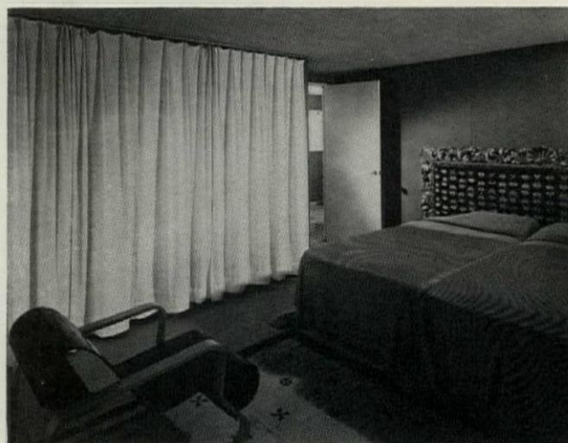
OWNER'S ROOM. The door is a 1 3/8-in. hollow casein-glued core, flush faced with gumwood.
