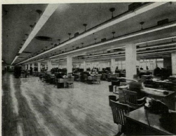
OFFICE SPACE in the administration building, lighted by fluorescent units providing 50 foot-candles at desk height.
