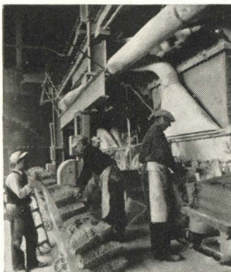
5 BAGGING. After various ingredients are added to regulate the set and working qualities of the plaster, it is ready for bagging.
