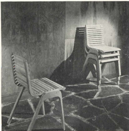
CHAIRS have plywood frames, sawn from thick plywood perpendicular to the laminations. The type shown here is non-resilient and can be nested in storage.
