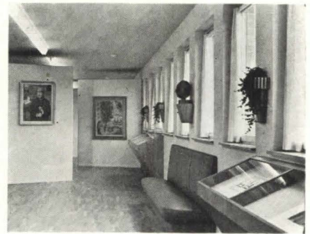
At Norrköping, ANGLED DISPLAY PANELS reduce reflections that occur when displays parallel the light source.
