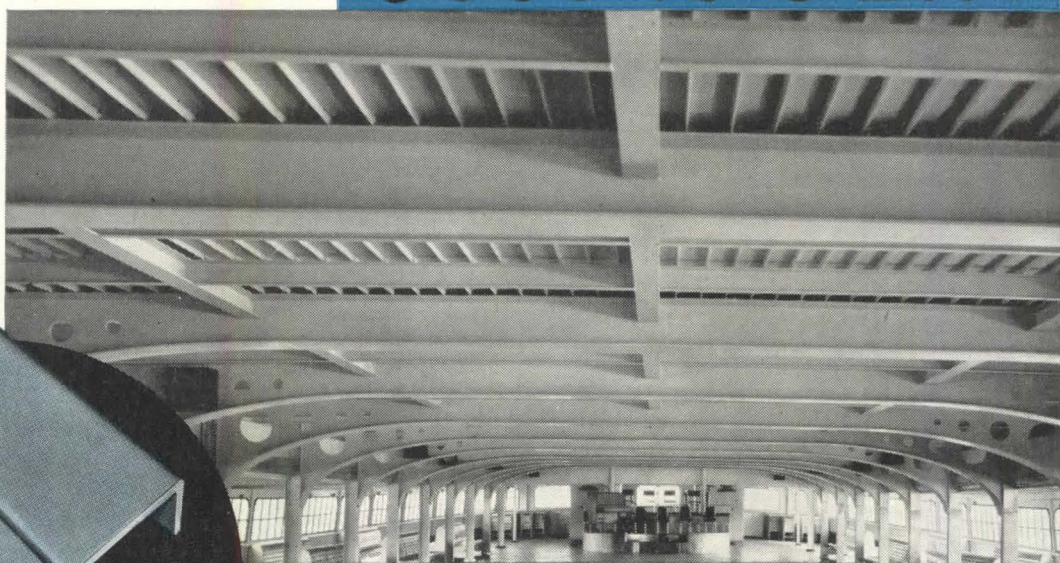
The Decks of the "Delaware Belle", new Wilson Line Excursion Boat, are of Mahon Steel Deck rolled from Yoloy.
