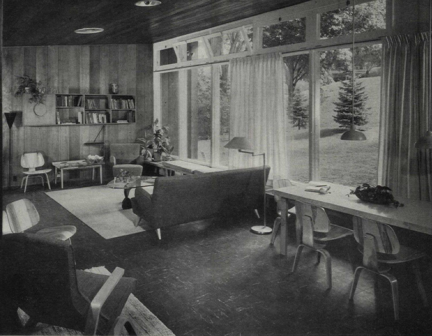
LIVING ROOM, toward southern window wall (large, fixed glass panes with ventilating transoms above); the ceiling and far wall of the room are of redwood, echoing the exterior wall finishes; asphalt tile is used for flooring. All upholstered furniture is covered with a dark blue herringbone tweed; furniture is light wood. The lowered light fixtures at right bring light down on the dining-work-play table. The room is planned and the furniture arranged so that several activities can take place at once—talk at the far end, music playing by the storage-wall units at left, eating or games around the big table at right.
