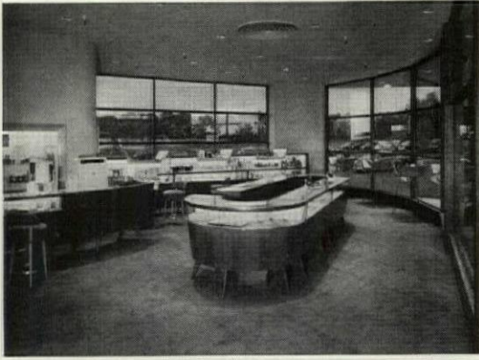
A TOILETRIES: Southeast corner. Painted plaster walls; lacquered display case frames.
