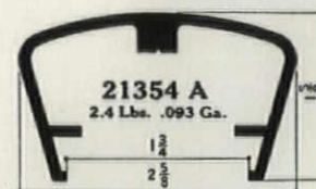
Nickel silver extrusion from Anaconda die 21354A forms handrail over nickel silver balustrade at rear entrance.
