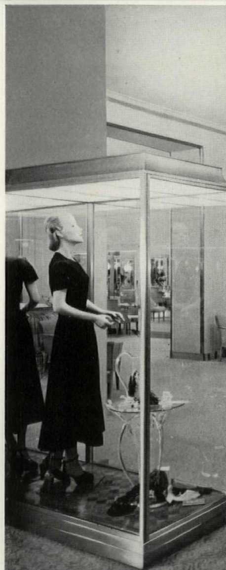
Display case frames are nickel silver and include extrusions from Anaconda dies 2917A and 13037A.
