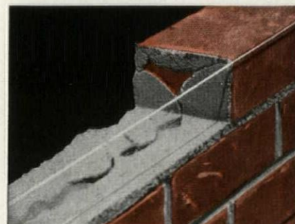
Even when mortar is spotted on both corners of the brick, slushing will not always fill the voids.
