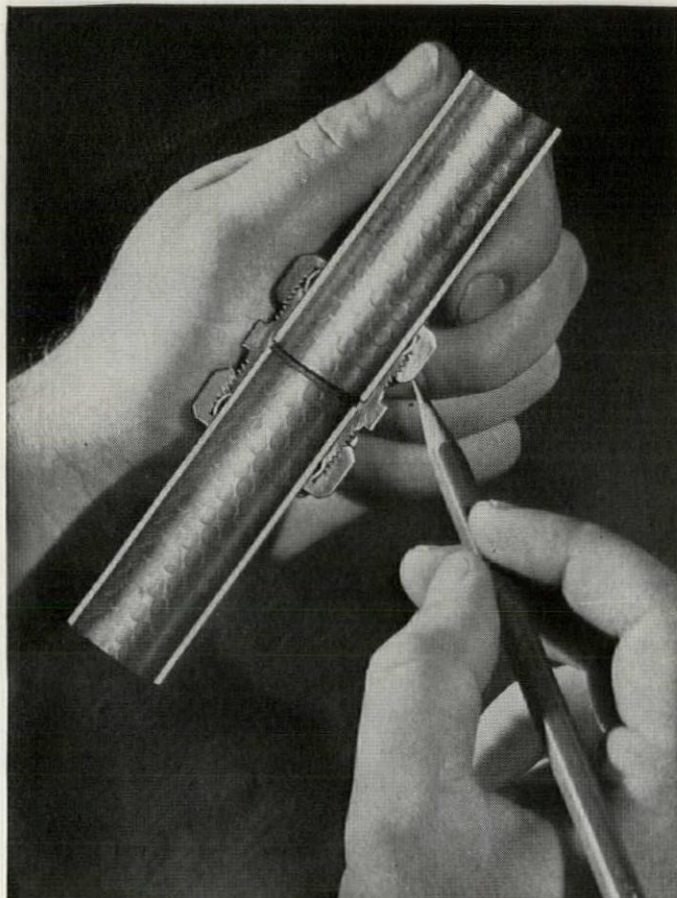
Cutaway view of compression coupling. Due to design of this coupling, there are no corrosion-inviting threads necessary on ELECTRUNITE E.M.T.—yet strong, water-tight joints are made quickly and easily with only a wrench or pliers.
