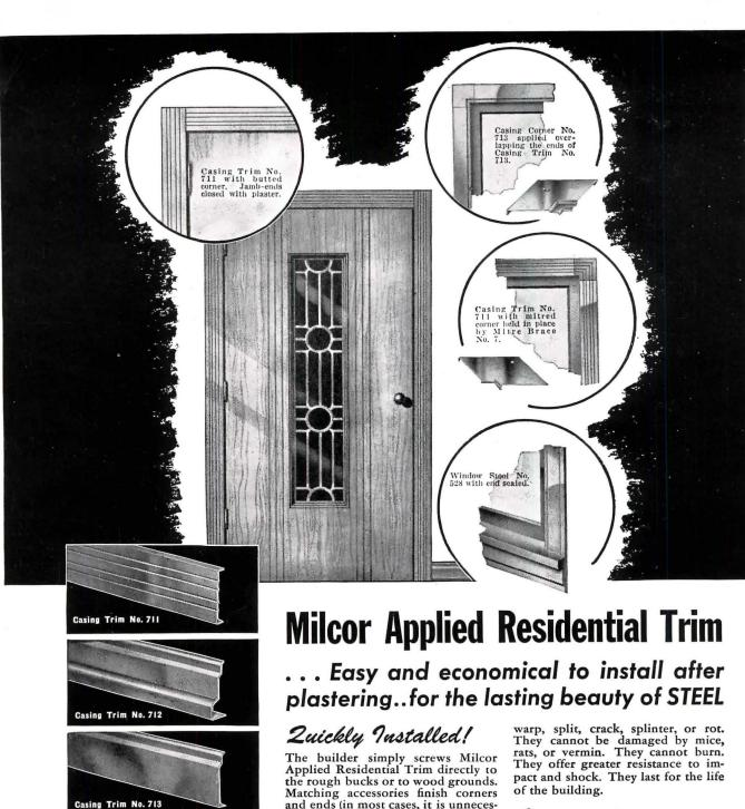
The builder simply screws Milcor Applied Residential Trim directly to the rough bucks or to wood grounds. Matching accessories finish corners and ends (in most cases, it is unnecessary to mitre or cut casings to exact length) — or you can butt, cope, or mitre at corners. To reduce painting time and costs, Milcor Applied Casings and Trim come with a rustinhibitive primer coat of paint.
