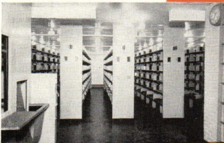
Bracket Stack with Hinged Open Bar Shelves and Wide Ends. Stack Aisle Light Reflectors and Stack Tier Conveyor Station. Howard University Library, Washington, D. C.
