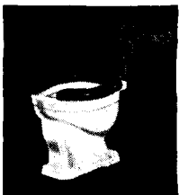
RAJAH VITREOUS CHINA FLUSH VALVE CLOSET —For 12-in. roughing-in. Round front washdown bowl, 1½-in. rear spud. B-6550 (illustrated).
