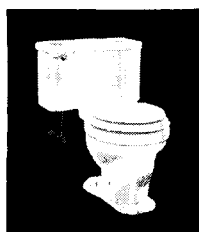
DUKE VITREOUS CHINA CLOSETS —For 12-in. roughing-in. Close-coupled, washdown, syphon action combination. B-6430 (illustrated).
