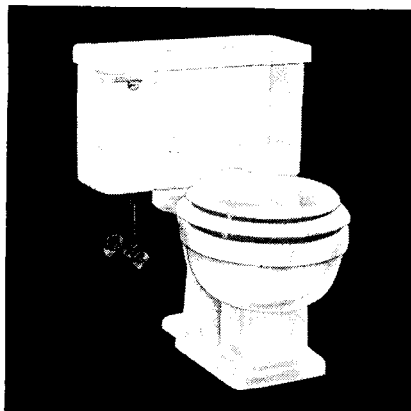
CARLTON VITREOUS CHINA CLOSETS —For 12-in. roughing-in. Full syphon jet free-standing unit. B-6400 (illustrated) close-coupled combination with regular, extended shelf bowl. Also available in elongated front extended shelf bowl model.
