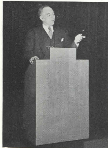
Above and below—a well lighted rostrum is a needed accessory for any auditorium. In this rostrum, two 8-watt miniature fluorescent lamps illuminate the speaker's notes and cast a pleasing glow on his face. A silent, electric timer paces his presentation and turns on an illuminated warning when the time is exhausted. A switch card on a retracting reel permits the speaker to signal the slide operator, even if he walks away from the rostrum. In this custom-built rostrum, a motorized elevating system raises or lowers the stand to suit the speaker's height.
