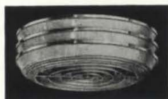
No. 3278 11 1/2" Dia. 3 1/4" O.A. 275W No. 3280 14 1/2" Dia. 4 1/4" O.A. 300W FINISH: Silvermat. Concentric Metal Louvres Baked Satin Aluminum. Punched for mounting on either 3 1/4" or 4" outlet box. Made of Aluminum.
