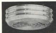
No. 3279 11 1/2" Dia. 3 1/4" O.A. 275W No. 3280 14 1/2" Dia. 4 1/4" O.A. 2-100W FINISH: Silvermat. Concentric Metal Louvres Baked Satin Aluminum. Purchased for mounting on either 3/4" or 4" outlet box. Made of Aluminum.
