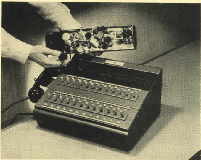
Figure 1—patient initiates conversation by pressing call button (below, left). Figure 2—master station combines built-in amplifier and double-throw cam keys to increase room station capacity and reduce size of cabinet (below, right). Figures 3 and 4 (center and bottom) illustrate the eight stations of the system and a conventional conduit layout.
