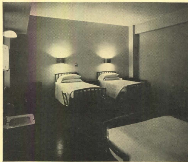
Figure 4—many architects prefer to dispense with ceiling fixtures in patients' rooms; the upward component of light from the bed lamps supplies the general illumination. George Washington University Hospital, Washington, D. C.
