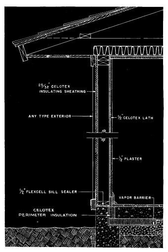
"U" value of this wall is 0.15 with wood siding and plastered interior
