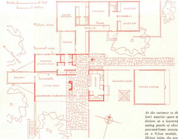
At the entrance to the house (two photos below) exterior space is defined by such various devices as a louvered wood fence and alternating panels of obscure and clear glass. The post-and-beam structural system was laid out on a 9-foot module, allowing direct use of 10-foot joists, the overlapping providing effective tie. Posts are 4 x 4's and beams, 4 x 14's. Photos: Richard Garrison
