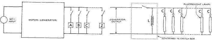
frequency (Figure 4), and the Group Operation Principle is employed. The auxiliary equipment is not designed as a oneor two-lamp ballast, as generally used today, but is arranged for the entire group controlled by a single wall switch. Much of the auxiliary can then be enclosed in an acoustically-treated wall switchbox.
