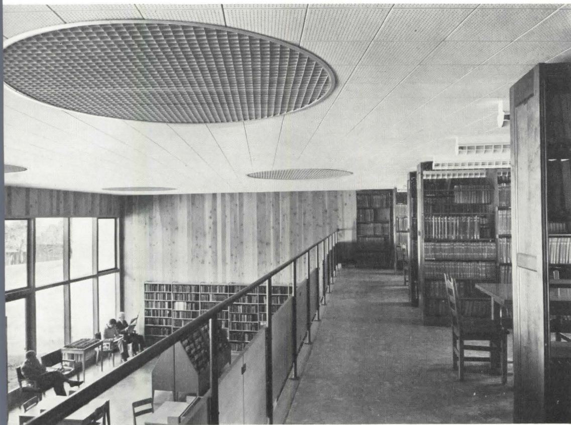
The warm tones of the cedar-board walls and neutral, tan-gray of the rubber-tile flooring set the muted color scheme of the interior. As a foil, the major steel beams are painted bright tile-red, while cross-beams under the mezzanine (right) are bright blue. Acoustic-tile ceiling is off-white. (SELECTED DETAIL, mezzanine railing, page 143)
