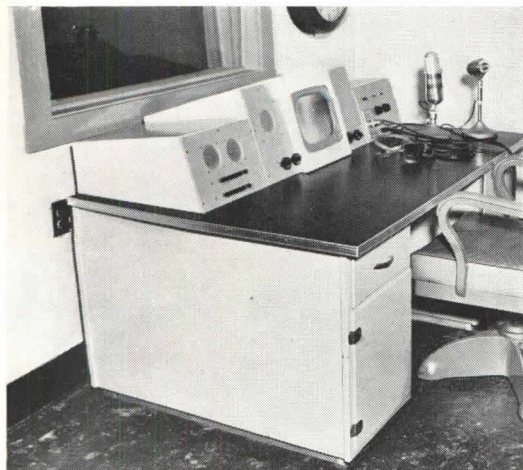
Announcer's console at WAAM, Baltimore (left); switching unit of video-control equipment (right).
