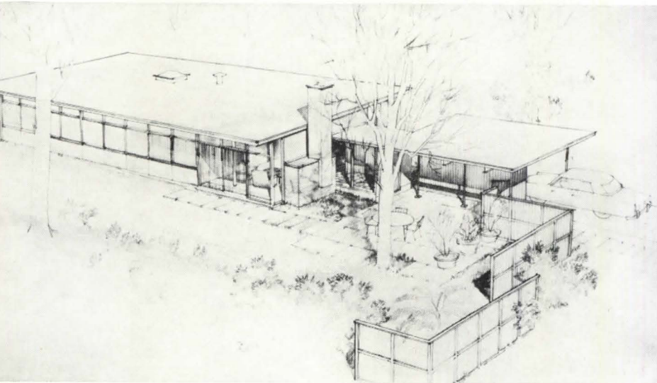
Ford and Robertson emphasize wall and partition flexibility that is possible through lift-slab construction for roof (below left). Very economical for projects of 50 or more homes, lift-slab can be built for about $1.35 per sq ft. Partitions easily changed to suit family needs.
