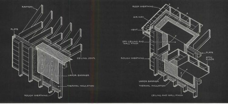
Figure 3—Vapor barrier at junction of attic floor, roof, and side wall in unfinished attic. Vapor barrier is extended from top of wall and continued along underside of attic floor before ceiling lath is applied. Note lap made on wall plate.
