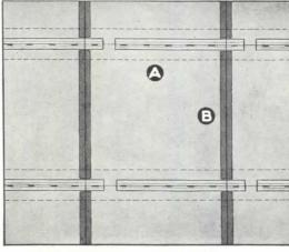
3 Supporting splines (A) are parallel to furring and continue through tile joints. Fiber cross splines (B) are used for leveling. They are no stapled, making installation still more economical.
