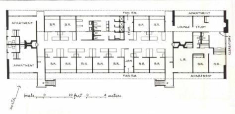
Typical dormitory (above) is constructed of wood, stone, concrete, building tile, bar joists, plywood, and asbestos cement.
