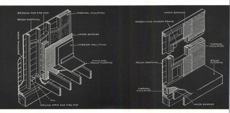
Figure 1-Vapor barrier at side wall where joists abut. The vapor barrier must always be continued down to the sill and nailed or stapled firmly so that no moisture leaks can occur at that point. Where joists abut the wall, it is necessary to reinforce the vapor barrier between the joists by nailing or stapling it to a nailing strip placed across the stud space just at the tops of the joists and then carrying it down to the sill.
