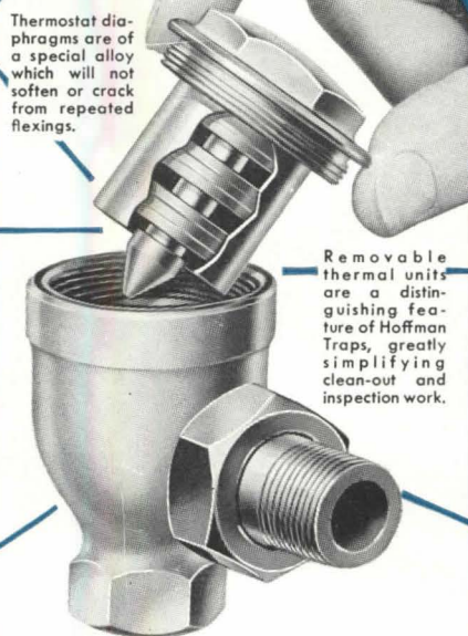
No. 8 Cap. to 490 lbs. cond. per hr. Max. Press.—50 lbs.
