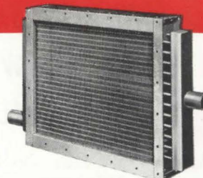
TYPE "HD" Coils—Heavy duty type for steam pressures up to 300 psi; temperatures to 500° F.
