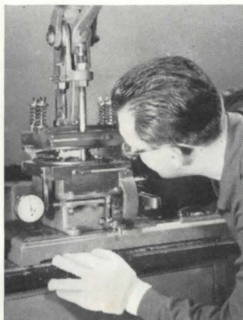
The ability of Kentile's top-grade raw materials to flow properly during calendaring is measured by a Mooney Viscometer.
