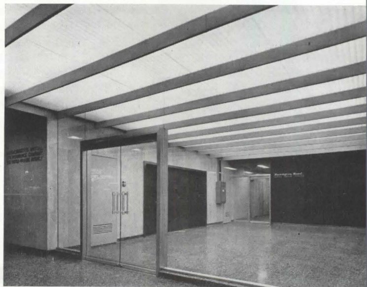
Figures 2 and 3—a new form of luminous ceiling employs arched sheets of acrylic plastic in metal frames resting on criss-crossed bars of perforated metal with glass-fiber packing for acoustic treatment (below). Metal frames are hinged and drop open to permit access to lamps and easy cleaning of plastic (below right).
