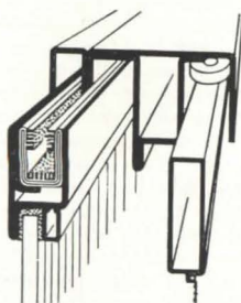
HEAD OF DOOR is weathertight with mohair pile that provides continuous weatherseal protection in top channel guide of door.
