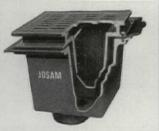
10 Josam Series No. 5250 Floor Drain with bolted top section, removable sediment bucket and heavy duty grate.
