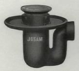
Josam Series No. 200 Floor Drain with integral drum-type "P" trap and adjustable strainer.
