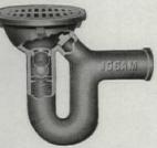
Josam Series No. 810-V combined Floor Drain and trap with ball type backwater valve and internal brass cleanout.
