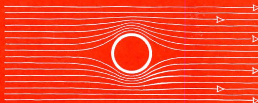
Figure 21— increase in flow speed around an obstacle.
