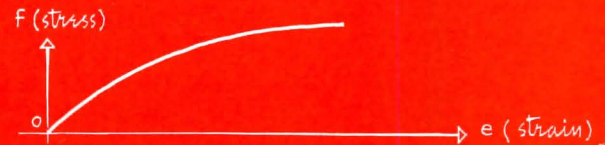
Figure 7—stress-strain diagram for concrete.
