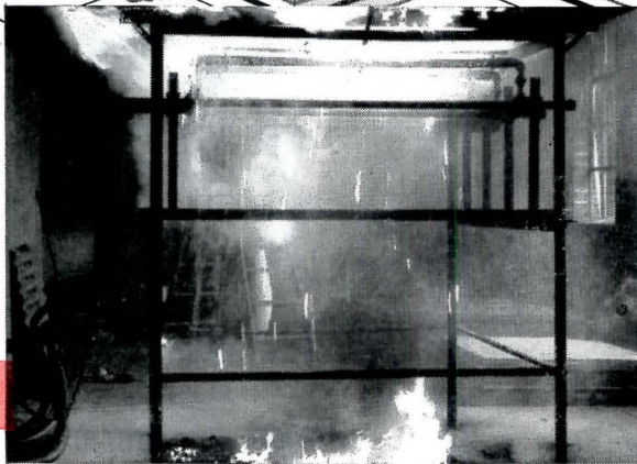
At the Carey Research Laboratories, this fire test of a conventional-vapor seal, with insulation and built-up roofing over steel deck, showed the dripping of asphalt from the vapor seal igniting as 1800° of heat builds up under the roof construction and melted bitumen flows through the joints in the deck.
