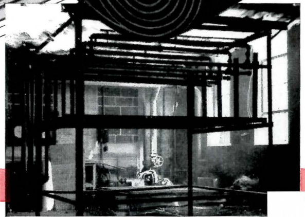
Fire test of conventional-type built-up roof with new Fire-Chex 1-ply Vapor Barrier over the steel deck (see diagram). Here you'll note a complete absence of any dripping material and only slight burning of gases. Practically no fuel is contributed to the fire by vapor barrier.
