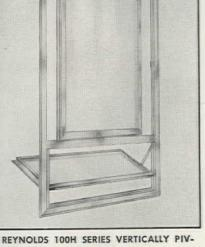
REYNOLDS 100H SERIES VERTICALLY PIV-OTED WINDOW used in Pacific Mutual Building. Provides minimum air infiltration, positive locking. Revolves easily for washing from the inside. All welded frame construction. Self-draining-
