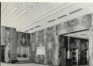
Line-O-Flo Ceiling Diffusers in lobby and court room areas quickly equalize temperature differential between supply and room air, preventing stratification and eliminating drafts. Combine readily with light fixtures.
