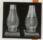
After 24 hours, note how much water has gone into and through the non-waterproofed mortar, and how little water has gone into or through the Brixment mortar.
