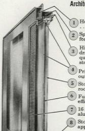
Hollow-type aluminum extrusions for maximum strength . . . 63S-T5 alloy, minimum thickness .062".
