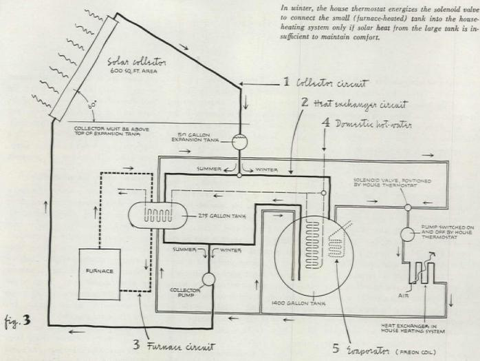
I-Collector circuit; pump on when sun shines.
