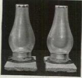
Prepare two slabs of mortar, one with Brixment and one with ordinary lime - and - cement mortar. After mortars have hardened, seal a lamp chimney to each of the mortar slabs, using wax or candle grease, and fill with water.
