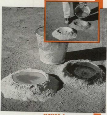
Pour out a pile of Brixment and a pile of ordinary cement and lime. Make a crater in the top of each pile. Fill each crater with water. Note how the cement-and-lime mixture absorbs the water immediately. Note how the waterproofed Brixment holds it.
