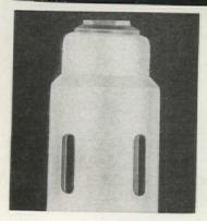
SLOTTED-NECK construction is an original ABOLITE feature! It keeps lamps cooler (40° cooler on a 1000 Watt lamp) - increases lamp life-reduces maintenance. ABOLITE SLOTTED-NECK reflectors keep dirt and dust on the move - they eliminate grime accumulation and
