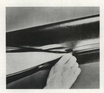
Thermal insulation on pipe and ducts can be protected by new-type, prefab Krene plastic cover. Cover is wrapped around insulated pipe and closed by pulling slide fastener which locks preformed edges. End joints are wrapped tightly with Krene tape. Will cover pipes from ½" to 33" in diameter and in lengths up to 100". Miracle Adhesives Corp., 214 E. 53 St., New York 22. N. Y.
