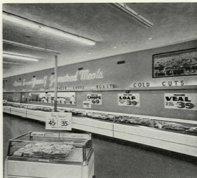
Acme Supermarket in Shoppingtown, DeWitt, N. Y., features a modern, year-round Carrier air conditioning system. Peripheral ducts carry cooled air from a 30-ton Weathermaker, warm air from two gas-fired duct-type unit heaters.
