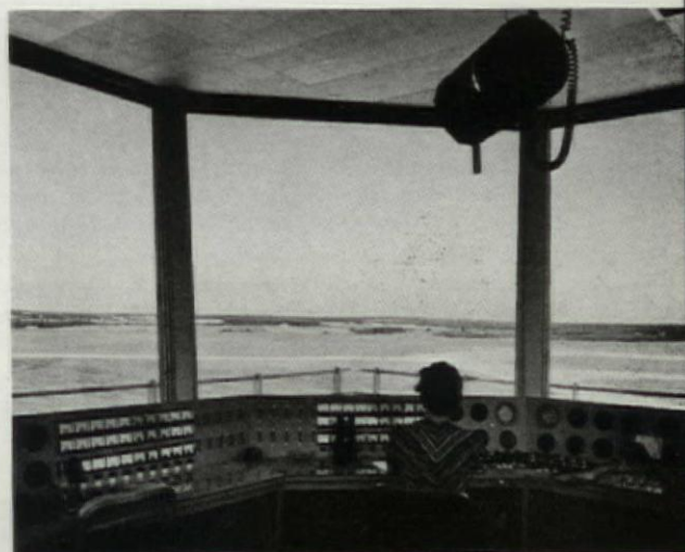
The control room is exceptionally well insulated for obvious reasons—acoustically treated; double glazing, separated by a 4-in. air space (outer pane, of heat-absorbing glass); acoustic pan ceiling; and heavy carpeting. Roof is of stainless steel to reflect heat; and stainless steel mullions were used to minimize obstruction to view.
