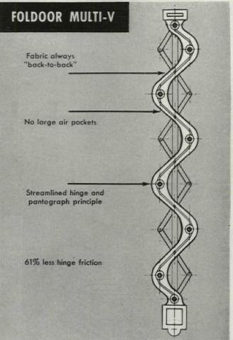
more working metal per foot of opening with less dead weight. What's more, the same 16-gauge hinge is standard on all Foldoors regardless of size. Foldoor has the narrowest profile, too—a stack width of  $5\frac{1}{2}$ ". Streamlined pantograph action lets it stack into just  $1\frac{1}{2}$ " per foot of opening.
