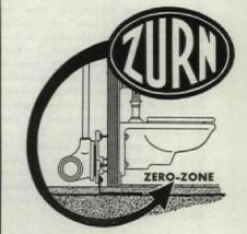
The ZURN ZERO ZONE is created by mounting off-the-floor plumbing fixtures on behind-the-wall ZURN SYSTEMS. This permits the highest degree of rest room sanitation to be attained and maintained. All major plumbing manufactures make fixtures to fit the ZURN SYSTEM.
