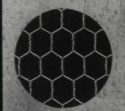
1. Keymesh woven wite galvanized reinforcing lath-applied over the gypsum or insulating lath on the entire ceiling; for highest quality, over all walls; too. This netvork of multidirectional reinforcing ncreases strength; increases fire afety 50%. Keymesh assures a inform thickness of plaster, and quards against cracks.
