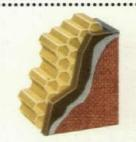
**Cross-section** of Kawneer honeycomb door showing complete lamination. Doors also available with ribbed aluminum skin only.
