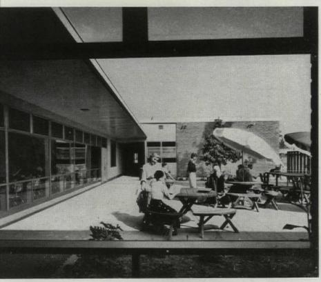
Opened sliding doors join lounge and main dining room (right). Structure is basically wood frame on concrete slab, grade beams, and caissons. Exterior materials include plaster, brick, and enameled-metal sunshades. Floorings are wood block or asphalt tile; acoustical tile is used on ceilings. Sash is aluminumprojected type. Parker, Zehnder & Associates, Structural Engineers; Bartlett & Berky, Mechanical Engineers; Sheldon W. Swickard, Electrical Engineer.
