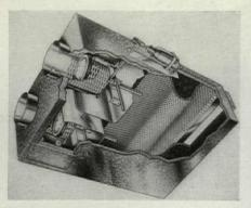
Felt-edged piston-type dampers regulate total air delivery, which remains constant
