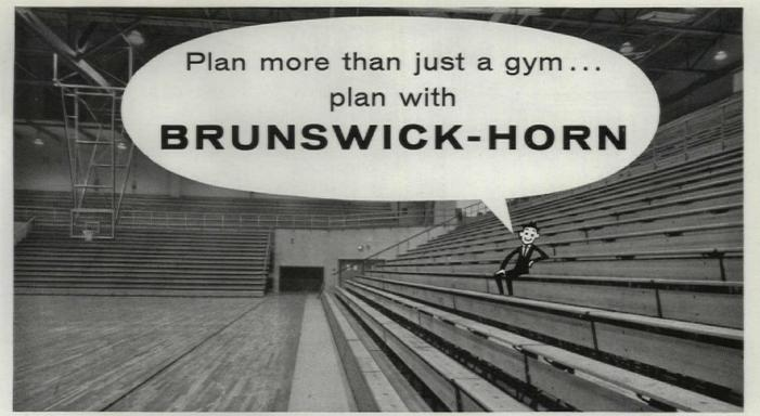
**Brunswick-Horn** Folding Gymnasium Seating locks secure opened or closed . . . cross-braced understructure stops sway or shake. In closing, foot boards tilt to spill litter on floor for fast, efficient removal.
