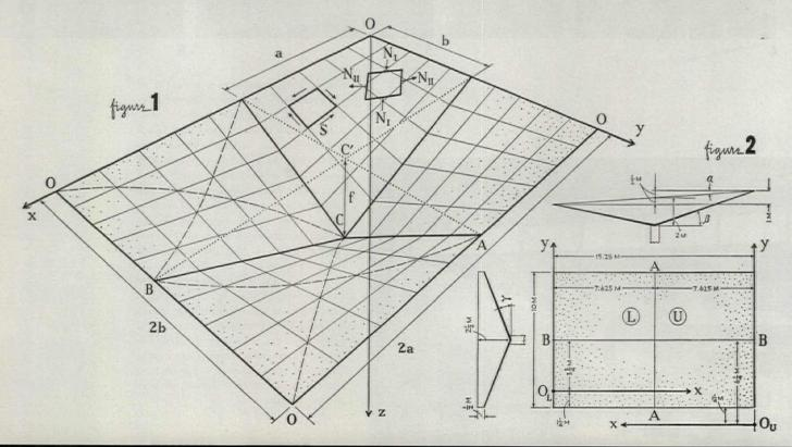
ground projection. Differences between the value of stresses obtained by this simplified assumption and those computed by accurate consideration of the real loads<sup>2</sup> amount to no more than five percent in this case.
