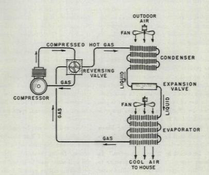
Figure 1-cooling cycle.
