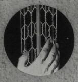
2. Keybead woven wire golvanized reinforcing lath with the precision-formed bead — applied at all outside corners — or zinc nose for outside applications. Open mesh of Keybead wings permits plaster to completely embed steel wires. Full, solid corners result. Available in standard lengths; easy to splice.
