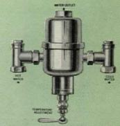
Powers Thermostatic Water Controller for regulating temperature of mulitple type showers, hydro-therapy and industrial processes. Capacities 22 to 125 gpm. @ 45 psi.
