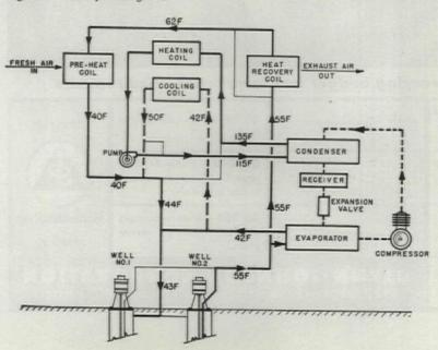
may be the availability of well water as a heat source and heat sink if the system is to be of considerable size. If the system is to be small—in which case an airto-air installation will be the simplest the principal consideration may be the severity of the winters in the location in question and, if in a northern location, the cost of electric energy for auxiliary heat.
