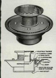
NO. 1205RA—Boosey Floor Drain for toilet rooms, mezzanines, second floor hospital areas, etc.: designed with an exclusive BOOSEY clamping device which assures positive sealing without puncturing the flashing material.
