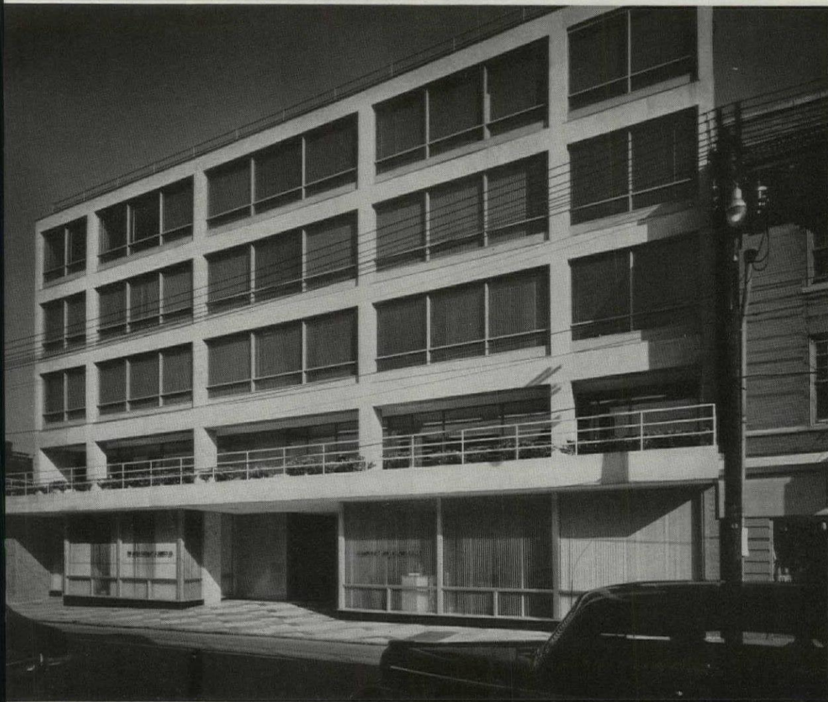
Intermediate projected sash were used for the windows, with green, heat-absorbing glazing. The storefront sections are aluminum. Photos: Joseph W. Molitor
