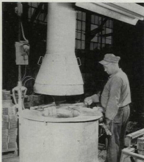
Figure 4—Exhaust hood for removal of fumes from a lead-melting pot (left). This is one example of local exhaust ventilation in industry.
