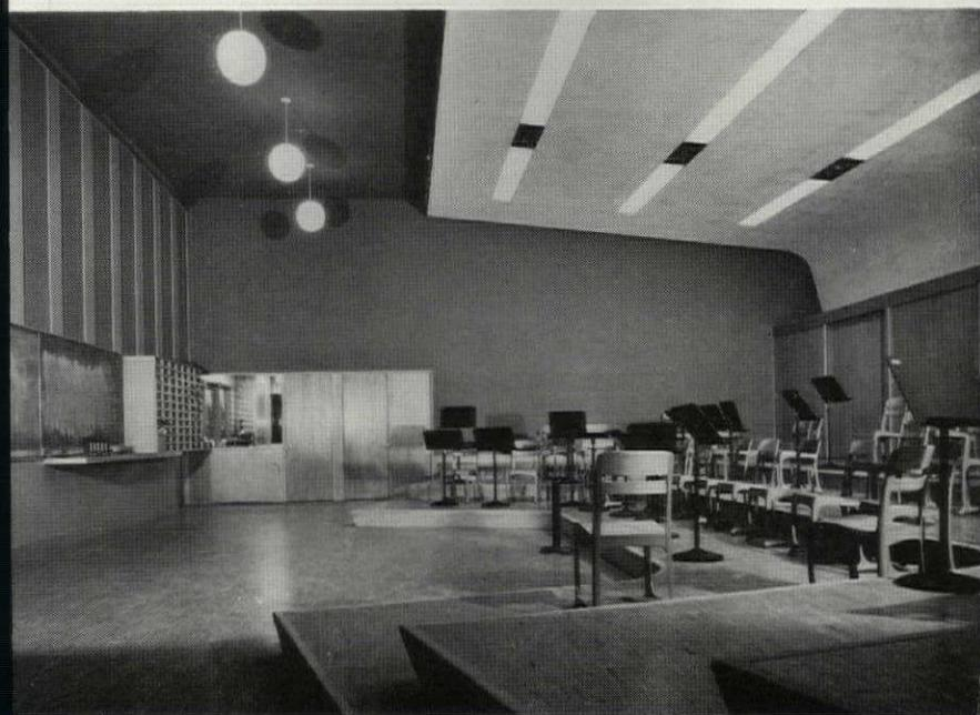
*Music building houses choral, band, and practice rooms, facilities for instrument repair, and uniform storage. Choral room (above) employs sound-absorbing blankets behind perforated-hardboard end walls. End walls, part of ceiling and wall above chalkboard in band room (left) are also acoustically absorbent. Instrument storage is at rear of room.*
