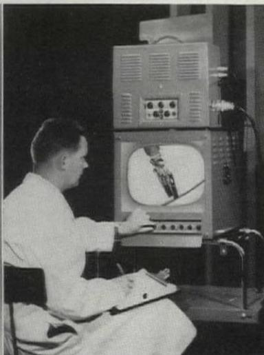
**IN LABORATORIES**, mills, factories, GPL ii-TV permits economical monitoring of remote or dangerous processes. Above, observer follows operation within a test cell. Other uses include plant protection and instructing workers.
