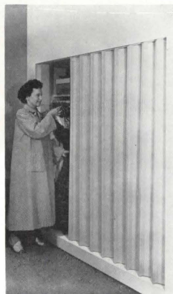
Lockable Folding Door: "Accordofold" (above)/nylon security latch permits locking/matching cornice also available/vinyl plastic over light teakwood insert in door body/door folds to 13% of its extended length in a 4 1/2" width that fits flush with standard 4" partition wall/in nine colors/self-lubricating nylon slides/mildew- and warp-proof/ American Bamboo Corporation, 171-06 Jamaica Ave., Jamaica 32, N.Y.
