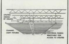
Typical ReynoCoustic applicationpanels and fiber glass backing rest on aluminum tees and angles. Marion Co. installation by Post Products, Inc., Boston, uses same method to suspend ceiling 3' below insulated roof. This space forms plenum for air conditioning system designed by Marion, engineered by Cobe & Foster, Inc., Manchester. System forces pre-filtered conditioned air into plenum at 24,000 cfm.
