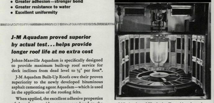
J-M's Accelerated Weathering Test subjected samples of dead level bitumens to repeated radiation, water spray and refrigeration. Results: Aquadam has approximately twice the ability of typical asphalts to retain its initial properties on exposure:
