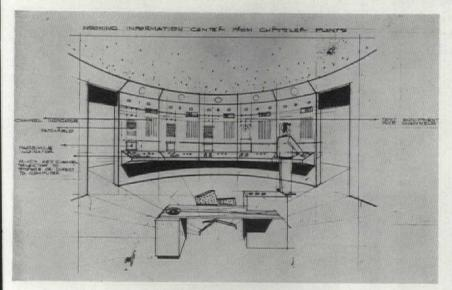
Incoming information is received at this center (left). Equipment includes channel indicators; facsimile indicators; punch-key channel selector to storage or computer; and testing equipment for channels. Consoles (below) provide electronic and magnetic storage of memory information for distribution to computers as well as sources other than Chrysler and outside telecommunication systems.
