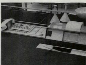
Machine (left) answers telephone while its owner is away. Cycle starts when telephone rings and receiver is automatically lifted. The owner's recorded voice requests the caller to leave a message. A wire recorder takes the message and the receiver is lowered when the call is ended.
