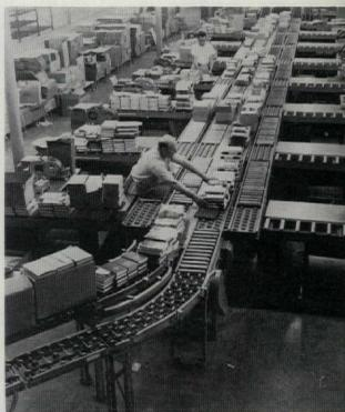
Dispatcher at book warehouse (left) places each order on weighing machine and marks shipping charge on invoice. From each side of dispatcher conveyor belts extend to the packing areas. From the packers, parcels move on belt to final inspection and stamping for postage charge. Kahn & Jacobs, Architects.
