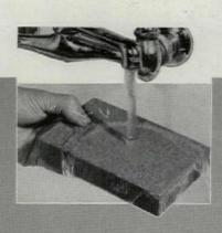
PERMANENT INSULATION — Beca Fesco Board has no wick-like action (as do fibr boards) it will remain dry under adverse job coditions. During an authenticated test in 24 hototal submersion in water, it absorbed only 1.4 by volume.
