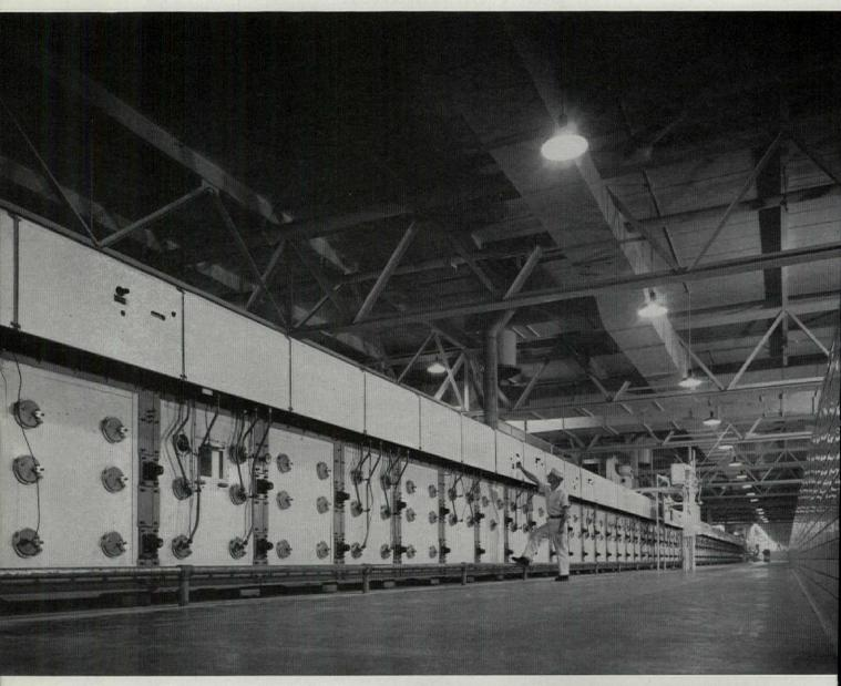
Sawyer Biscuit Company, United Biscuit Company of America, Melrose Park, Ill. Skidmore, Owings & Merrill, Architects-Engineers. In this handsome, long factory, crackers and cookies being baked travel continuously through nearly 600-foot-long banks of ovens, with no workers involved, except for the maintenance of the machinery. Exposed steel frame of the building is painted white; walls are gray, glazed brick.
