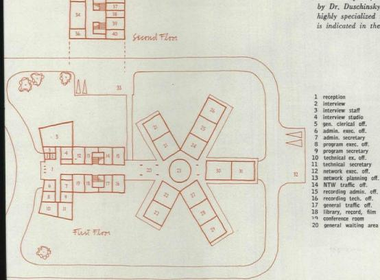
Schematic plan for a time-zone station, developed by Dr. Duschinsky, consultant. How one of the highly specialized recording rooms might appear is indicated in the drawing (above).
