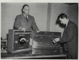
This flash- or flame-detection system (left) is triggered by means of photo-electric cells integrated into fire-control system. Commonly used as a personnel-safety measure, this system has been applied (as shown, left) to dangerous rolling-mill operations in the production of jet-propulsion powder.
