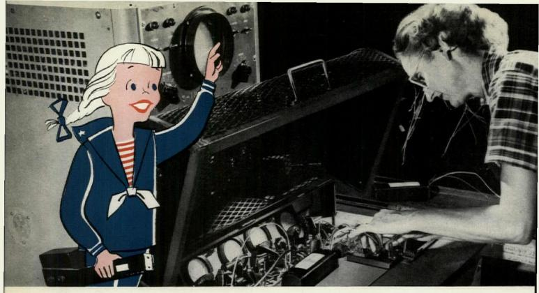
This electrical surge test is one of the 258 tests that every G-E ballast receives during the manufacturing cycle. This test subjects G-E ballasts
