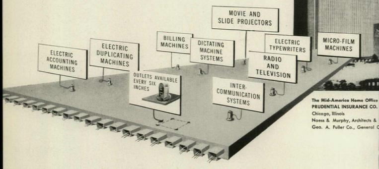
The new Mid-America Home Office of The Prudential Insurance Co. of America was designed with an eye toward the future. To meet the ever-increasing wiring requirements of modern electronic office equipment, architects Naess and Murphy prepared the structure to handle the highest electrical load of any office building ever built. To do this job easily and to permit power and telephone outlet changes and additions at minimum cost, Robertson Q-Floor construction was used.
