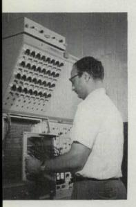
Electronic differential analyzer (left) in use at New York University College of Engineering. Problem has been set on panel. Knobs above are potentiometers that set various values for equations.
