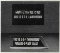
COMPARE the reflections of the upsidedown signs in the mirror of conventional plate glass (top) and the mirror of Parallel-O-Plate\* (bottom).
