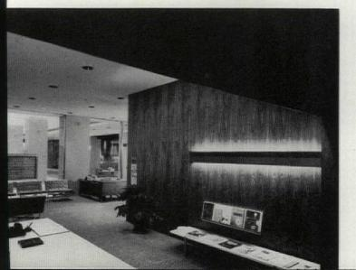
by IBM. In this area, the lighting changes to a geometric pattern of downlights recessed in the ceiling, affording both ambient lighting and highlights on objects displayed.
