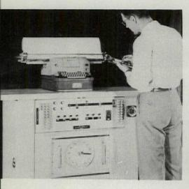
Automatic logger (above) tabulates essential variables, together with time of recording, on electric typewriter. Also produces punched-tape output which may be used to feed computers for automatic material-balance and yield accounting. Between tabulations at fixed intervals, logger can scan all inputs and if conditions are normal, no recording occurs. If conditions become abnormal, an audible alarm is sounded and a recording cycle is initiated.
