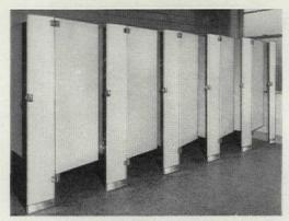
WEISART floor-braced style is especially popular for remodeling jobs, as well as new construction. Note clean lines for easy maintenance, and the absence of head rails. Rigid, sturdily constructed for years of trouble-free service. Choice of 24 oven-baked enamel colors. Brass hardware is chrome plated.
