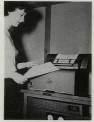
The world's fastest telegraph, the "High-Speed Fax" receives messages in facsimile picture form. The automatic recorder (left) cuts off and ejects the received message. High-Speed Fax is capable of sending messages at a rate of 3000 words a minute.
