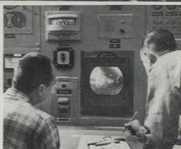
Interior of jet engine (left), being tested under various simulated speeds, temperatures, and altitudes, can be observed by TV circuit (below left). TV camera is trained on the combuster section of the jet engine to detect any possible defects which might develop during strenuous test. Control room (below) is part of TVA's large Johnsonville
