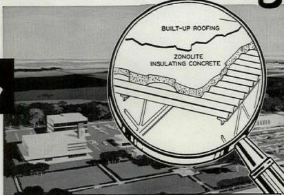
Important new development in corrugated metal deck. Here is artist's conception of Great Southern Shoppers Mart, Bridgeville, Pa. Zonolite Concrete was poured in place over corrugated metal. Zonolite pours on fast, cuts labor costs. Reduces insurance premiums as much as 1/2. Seamless, monolithic construction protects against "tardrip" should fire originate in under-areas. Mail coupon for free booklet.
