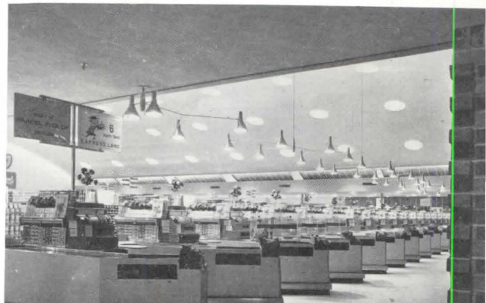
Flooring throughout is terrazzo; ceilings are surfaced with acoustical plaster. General Contractor was McLain Construction Company.
