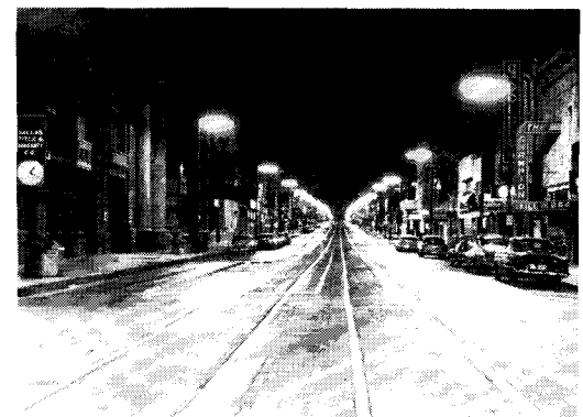
Figure 15—high-traffic business street in Dallas, Tex., with four fluorescent lamps (21,000 total lumens) per luminaire; 30-ft mounting height, 70-ft spacing.
