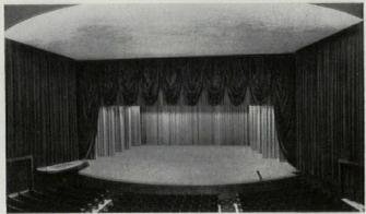
Take the Dade County Auditorium, Miami, Fla., for example. The electronically controlled Multo-Form contour curtain, designed and installed by J. R. Clancy, permits an infinite variety of openings. Contours for the entire show are programmed in advance.
