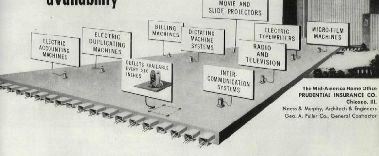
When you build with Robertson Q-Floor you assure a long and useful life for your building since you will have provided for any conceivable amount of office automation. The large steel cellular raceways in Robertson Q-Floor, on six-inch centers, make it possible to run wires for electrical and telephone outlets to any point in the building quickly and inexpensively. Thus, no matter how many electrical devices are added or moved, the Q-Floor building will have adequate electrical facilities.
