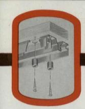
... Adjustable header with continuous strips Mohair pile running full length.
