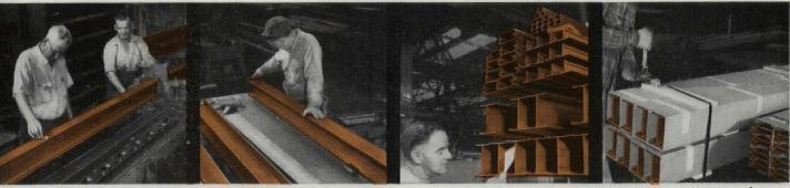
**STRAIGHTENING PROCESS** involves drawing shape through a second die. PAINSTAKING HAND WORK assures that dimensions are micrometer-perfect. **QUALITY CHECK** is made at factory of four shapes produced by Chase. CAREFUL PACKAGING makes sure shapes reach building in flawless condition.
