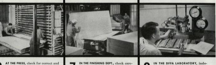
IN THE FINISHING DEPT., check carefully for grade and appearance. Check accuracy of dimensions and thickness. Apply grade-trademarks.
