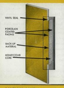
PANELFAB PANELS are available with porcelain facings in 8 types—sizes up to 4' by 10'; with aluminum facings in 3 types —sizes up to 4' by 24'.
