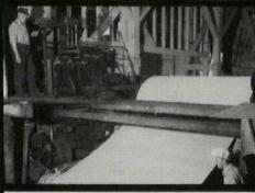
AT THE LATHE, veneer is checked for uniform thickness. This provides correct thickness of finished panel and permits optimum glue spread.
