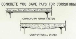
Diagram shows how Corruform stays level, saves about 20% or more in concrete over "flexible type" centering.
