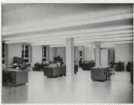
Here's an interior view showing a small part of the installation of Gold Seal Inlaid Linoleum. Actually, about 3½ acres of floor space are covered with this ½" burlap-backed "Veltone."
