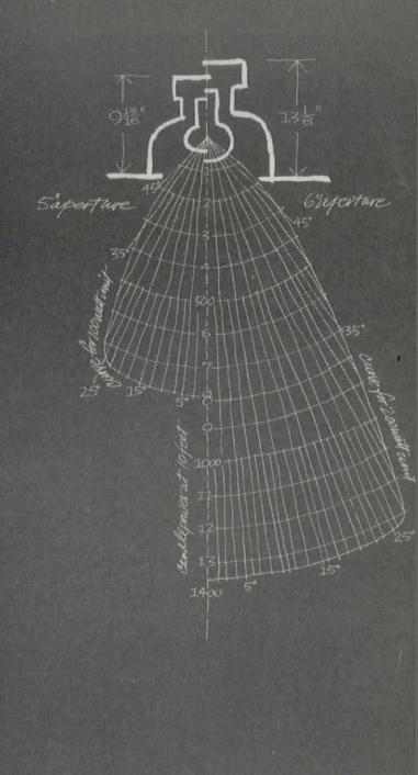
These E. T. L. distribution curves assure predictable performance of Gotham's recessed low-brightness alzak downlites. For data, write...
