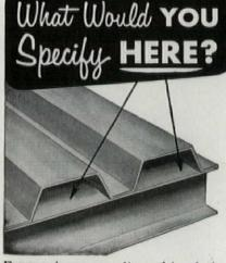
For maximum security and insulation, the end openings in metal roof decks and ribbed siding must be sealed. How to do this practically and economically has been the problem of architect and builder.
