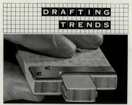
Magnified view of the laminated bamboo construction used in Post slide rules.
