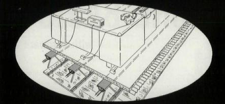
Wiring can be brought up through the floor at any point along the joists.
