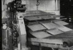
AT THE DRIER, veneer is checked for correct moisture content, which gives maximum dimensional stability and proper glue bond.
