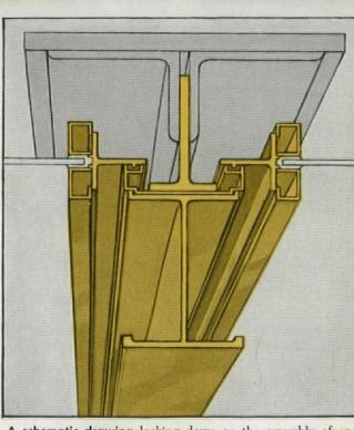
A schematic drawing looking down on the assembly of extruded shapes which compose the architectural mullions—and frame the fixed windows and bronze spandrels. The heavy Tshaped extrusion between the steel angles is used only in short lengths at each floor level (see photo, lower right) and transmits the weight of the bronze facing and windows to the structural steel framing.
