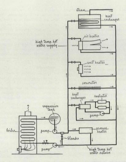
Figure 9—typical arrangement of an industrial HTHW system.
