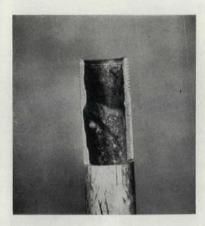
Galvanized-iron pipe perforated in six months. Area above and to right of hole has heavy copper plate. Circulating water had pH of 3.0 to 3.5.
