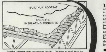
Zonolite concrete over corrugated metal...Diagram of roof deck just completed on huge shopper's mart in Bridgeville, Pennsylvania.
