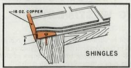
This edge for shingle roofs serves as a guide and assures alignment of shingles at end of every slope—protects the exposed edges of shingles.
