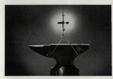
ADHERES WEATHERBAN Sealer bonds these metal discs, doesn't lose adhesion even when a 125-pound anvil is supported from them. Such positive, lasting adhesion means watertight, dependable sealing. Test WEATHERBAN Sealer yourself on stainless steel, aluminum, glass, stone or concrete.
