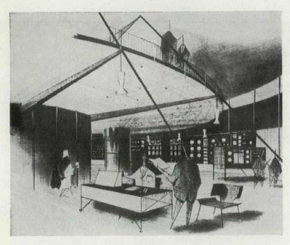
Hypothetical automated office building, developed by Irving Shapiro and Louis M. Naidorf, Architects. Machine floors such as the one above would contain central processing, printing, typing, and memory units and would occur in groupings at every sixth or seventh floor, as indicated in the exterior perspective. Plans at right are of executive and machine levels.
