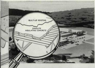
ZONOLITE CONCRETE OVER FORMED STEEL ROOF DECKS—Eberhard Faber Pencil Co., Wilkes-Barre, Penn. Another big structure with a permanent monolithic roof that weighs less, is strong, insulating, fire-safe. Arch.: Eyerman-Hoban & Sincavage, A.I.A., Wilkes-Barre, Penn.
