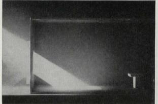
CLEAR GLASS — Actual photograph of "smoke box room" with its window glazed with clear glass. Note high concentration of light near window.
