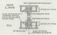
Figure 6-recommended clearances in using stops or moldings with glass. (Detail from Curtain Wall Seminar, New York Chapter Producers' Council; drawn by author.)
