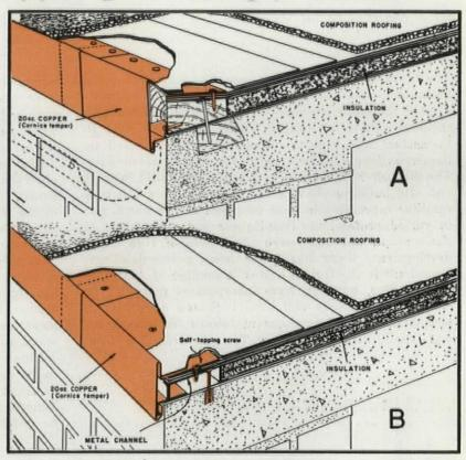
Edges for insulated built-up roofs. There are two problems. One is a firm and secure fastening for the metal so that it will retain its bond with built-up roofing. The other is construction to prevent horizontal shear at the margin of the relatively soft cellular insulating material. Figure A shows how to meet these problems with wood nailers—Figure B, with incombustible metal channels.
