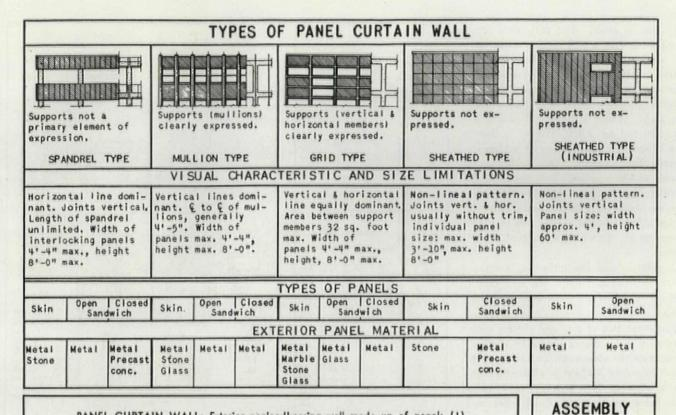
PANEL CURTAIN WALL: Exterior nonloadbearing wall made up of panels (1) attached directly to building structure with an adjustable attachment, or (2) mounted on supports (subframe), which in turn, are attached to building structure by adjustable attachments. Exterior surface of panels forms face of building; interior surface may or may not form interior finish.
