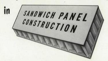
Between the skin, or outer face, and the core is the adhesive. Here is where you find the key to the life of sandwich panel assembly.
