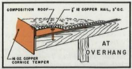
Copper edging has a 4" flashing flange, a 34" gravel stop, and a drip edge extending at least 14" below sheathing.
