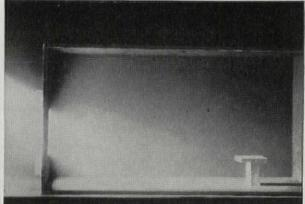
**DIFFUSING GLASS** — Smoke box photo — window glazed with diffusing glass. Note uniformity of lighting and its distribution to far side of room.
