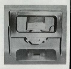
hushing chamber and mixing apparatus (above). Warm air and cold air are delivered through dual ducts at bottom and mixed according to thermostatic setting in bellows arrangement behind perforated cover. Capacities of basic unit range from 100 to 300 cfm. Buensod-Stacey, Inc., 45 W. 18 St., New York 11, N. Y.
