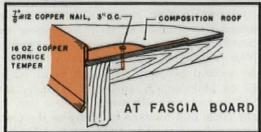
Same as edge for overhang, except that outer face is deeper for neat appearance and bottom edge is turned back to form a hem, canted outward to serve as a drip.
