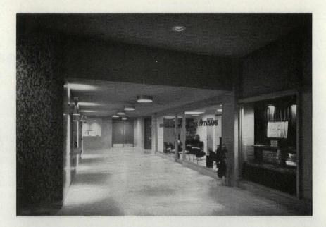
Exterior and interior color schemes were based on white, silver, and aqua blue, Porcelain-enameled panels at curtain wall are aqua blue outlined with aluminum; end walls, white brick; exterior columns at first floor and underside of entrance canopy, ¾" x 1½" aqua blue ceramic tile; lobby floor and shopping arcades (right), white terrazzo with blue-gray insert; walls of elevator shaft at lobby, Italian glass mosaic tile from pure white to dark turquoise.
