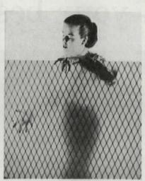
Metal-reinforced translucent plastic panels-using either aluminum or steel diamond-mesh-have high impact resistance (left). Sheets can be obtained in both standard and special fire-retardant types, in clear, and in five colors: blue, green, yellow, sky blue, and coral. Panels available in lengths of 8' and 10' and widths of 1', 2', 3', and 4'. Resolite Corp., Zelienople, Pa.
