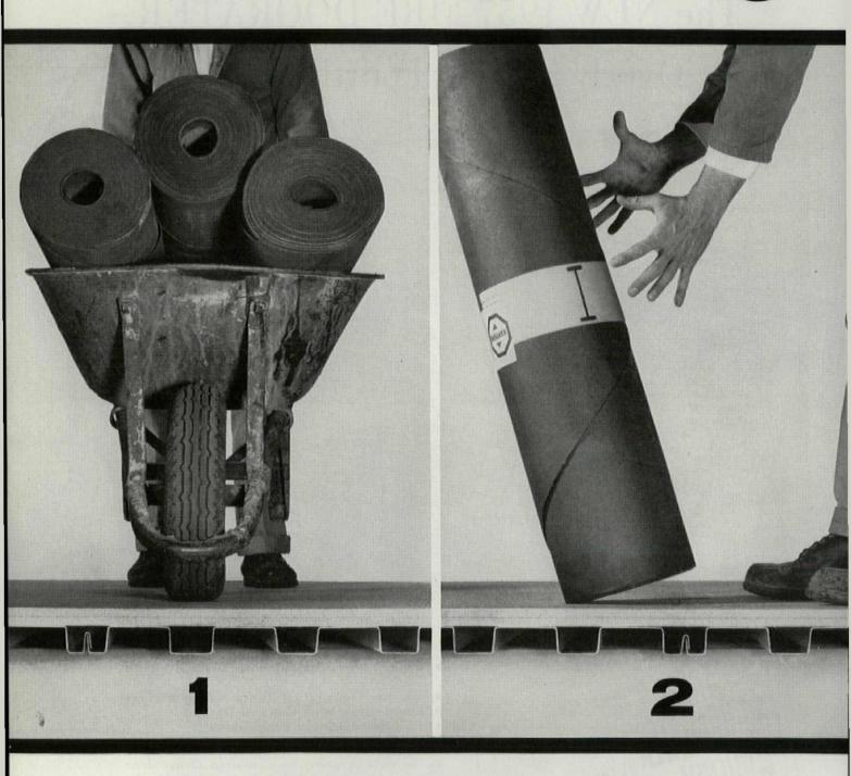
These tests can be made at any roof job: 1. BARROW TEST. Run heavily loaded barrow on line between support surfaces. 2. DROP TEST. From height of 12 inches, drop wrapped roll of roofing felt, letting edge strike insulation. 3. HEEL TEST. Kick the insulation sharply, at any point between flat support surfaces. In these tests, Insulite Roof Insulation will not crack, crush or break through. 1-inch Insulite Roof Insulation was used in tests illustrated.
