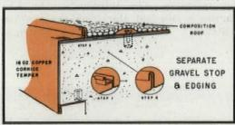
Edging for built-up composition roofing on a concrete deck, designed to show minimum of waviness or buckling. Facing strip is free to slide because of clinch lock seam at top and bottom. Standing seam at top is rolled toward outside and serves as gravel stop. Bottom seam is simple clinch lock joining fascia with stiffening strip for trim appearance and to provide a drip edge.
