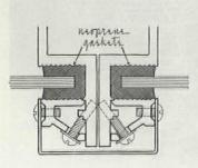
break, the same rubber gasket and aluminum frame can be reused to replace the light. Each gasket will expand or contract as necessary to accommodate movement of the glass skins, and long life is assured since neoprene has a proven re-
