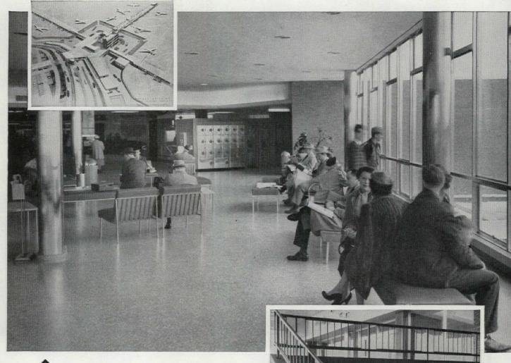
Functional and decorative use of stainless steel is shown in this section of the main waiting room of Cleveland Hopkins Airport Terminal Building. Stainless sheet was used for columns and lockers. Furniture bases were fabricated from stainless steel tubing. Architects, Outcalt Guenther & Associates, Cleveland, Ohio; General Contractor, R. S. Ursprung Company, Cleveland, Ohio.
