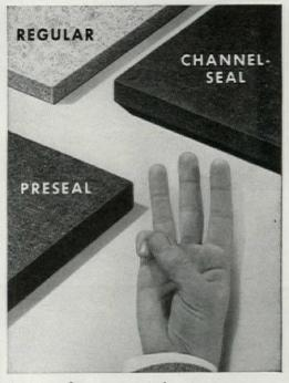
A type for every job requirement. PRESEAL: Asphalt-coated on both faces and edges for greater protection against moisture pick-up. CHANNEL-SEAL: Bevels on deck-side form network of channels for equalization of air and vapor pressure, providing extra protection against blistering and separation of felt and insulation, asphalt-coated. REGULAR: Uncoated Celotex board. Recognized standard where lowest cost insulation is required. All in a variety of thicknesses.
