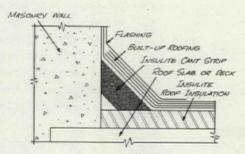
**Insulite Cant Strips** have long been accepted as the ideal angle-breakers at points where roof surface meets any vertical surface. Made in two sizes, 3"x3" and 4"x4".
