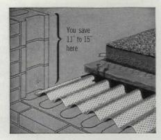
5-INCH SYSTEM. A suspended ceiling system usually requires 16" to 20" in depth. Only 5" deep, the Structur-Acoustic system saves 11" to 15" in wall height, saves thousands of dollars in materials and labor.
