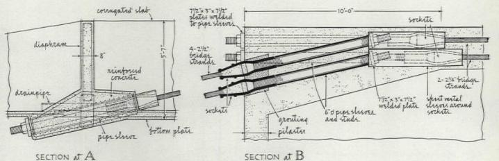
the roof slabs; before removal, each cantilever shell was jacked and raised from the forms to accommodate the anticipated elongation of the strands-about four in. elastic strain per unit. Wood forms on tubular scaffolding was used for the three-ft deep corrugated - slab floors of the center section. Suspender rods, 11/8 in. and 21/2 in. diameter, hold the second and third floors respectively from the anchorage above.
