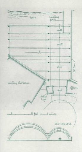
In bold sweeps recalling the waves of the ocean, these concrete shells now link a number of formerly unconnected structures on the beach. Purpose of the arched roof was to provide a cool, airy sun shelter. Two small enclosures provide the entrance-control points for the club: one for offices, the other for lockers and keys.
