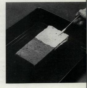
pellency could be achieved without interference with the normal "breathing" of these porous substances. Soon after World War II, a series of silicone products became available to exploit this performance.
