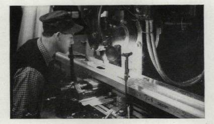
Albro milling machine routes out channel for door hardware made of Alcoa Aluminum.
