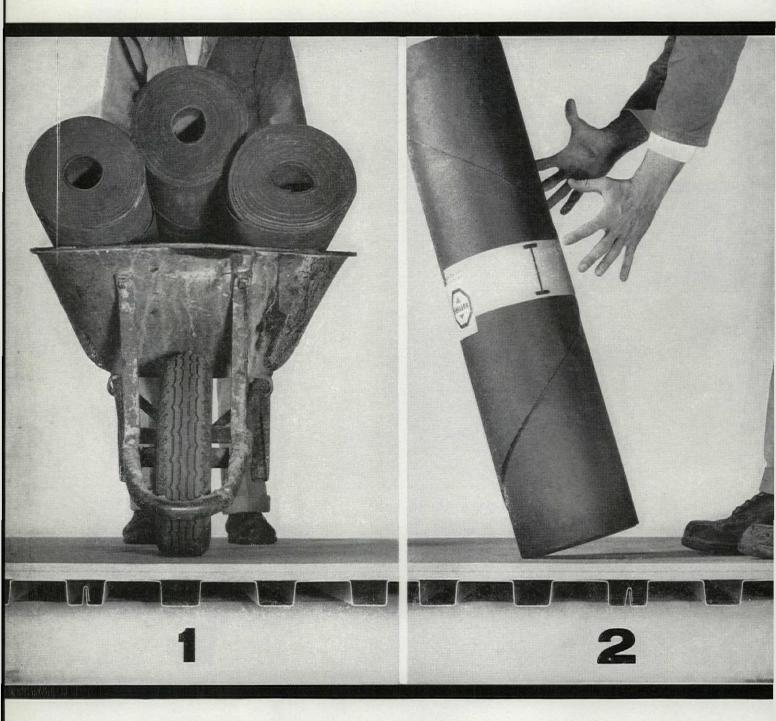
These tests can be made at any roof job: 1. BARROW TEST. Run heavily loaded barrow on line between support surfaces. 2. DROP TEST. From height of 12 inches, drop wrapped roll of roofing felt, letting edge strike insulation. 3. HEEL TEST. Kick the insulation sharply, at any point between flat support surfaces. In these tests, Insulite Roof Insulation will not crack, crush or break through. 1-inch Insulite Roof Insulation was used in tests illustrated.
