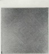
Decorated Ceiling Tile: "Temlok Tile" in "Diamond" design/ beige imprint over white ground/ 12"x 12", 1/2" thick/ tongue-and-groove joints permit blind-nailing, stapling, or cementing/ Armstrong Cork Co., Lancaster, Pa.
