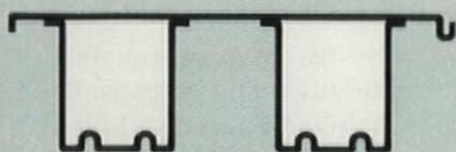
SECTION M2-7.5 CEL-BEAM DEPTH 7 1/2"
