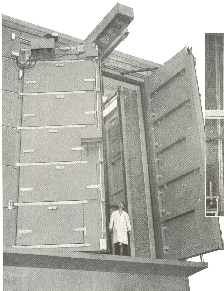
HUGE TEN-PANEL double leaf Jamison Sound Reduction Doors in test cell built for hypersonic combustion tests. (right) In the event of explosion, blowout panels are forced open to prevent personnel and cell structure damage.
