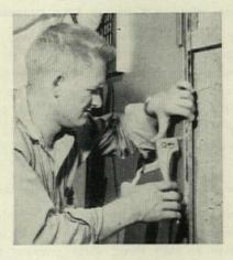
high as 1600 lb, procedure furnishes tight, vibration-proof clinch. Made in five different combinations of mandrel and head types: break stem mandrel, where mandrel head is held in rivet after setting; break head mandrel, where mandrel head falls clear when rivet is set; domed head, giving low head profile and extra clearance; countersunk head, where flush appearance is desired; and new "Imex" Pop rivet, a sealed-end rivet.
