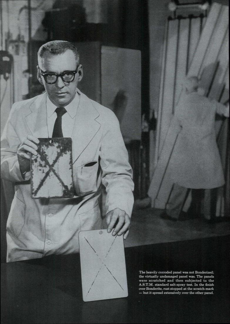
Continuous 8-day salt-spray test proves prime advantage of Milcor steel roof deck
