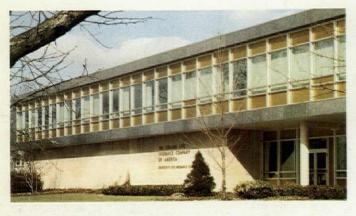
**HEAT ABSORBING PLATE**—For reducing the initial cost of air-conditioning equipment and its operating cost, L·O·F makes two kinds of ½"-thick polished plate glass: Heat Absorbing and Parallel-O-Grey. L·O·F Heat Absorbing Plate Glass has a pleasing blue-green color. Parallel-O-Grey has a neutral grey tone that does not change the color of objects seen through it. Both offer some relief from sun glare; Parallel-O-Grey to a greater degree. Comparison of solar heat transmission is as follows:
