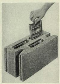
foil insulation. Insulators are sealed in as wall is built; a cap is placed over air cells between each row of blocks. Tests at Armour Research Foundation also reveal blocks possess high soundproofing capabilities.
