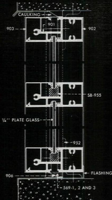
You can frame windows and glass-clad walls completely with the related components of the new PITTCO "900" series. It is provided with a drainage system. All members are aluminum; all fastenings are concealed; all glass is held in neoprene strips and recessed to increase daylight opening. And the clean beauty of every line is strikingly apparent. For details, consult your PITTCO Metal Representative.
