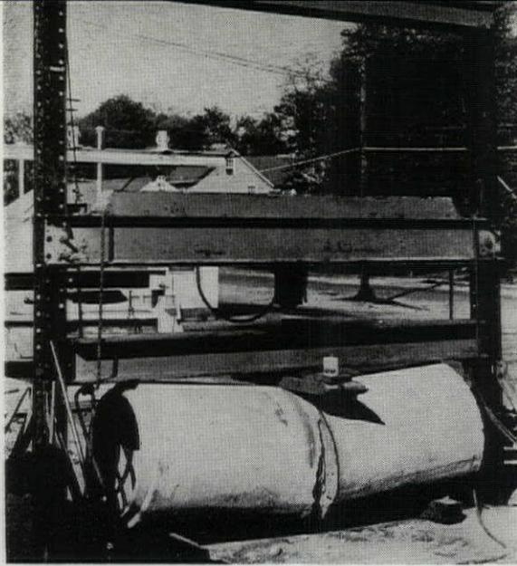
*Figure 2—Two sections of 40" diam. reinforced-concrete pipe, joined with epoxy adhesive, subjected to load test (above). Break occurred at approximately 34,000 lb. Close-up view (right) shows break to be outside of weld.*
