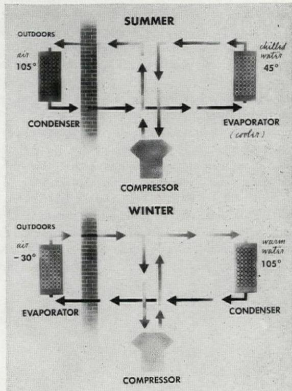
Figure 4—Heat-pump compression cycle at Flick Reedy Corporation.
