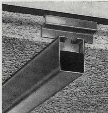
Standard high speed T-clips lock quickly into slotted box sections. Resistance to uplift pressures at the clip have been tested in excess of 450# at the clip, or 60 psf, meeting hurricane wind uplift ratings. Vertical load tests are certified by Pittsburgh Testing Laboratories and Ohio State University Engineering Experimental Station. Clips are completely enclosed at the plank joints—reducing thermal transfer through the roof deck.
