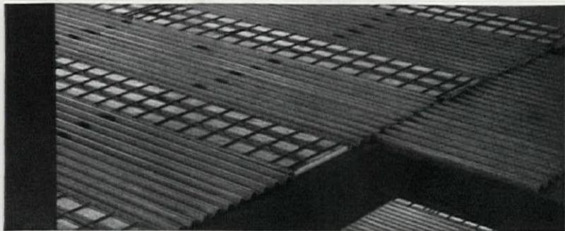
**TUF COR AND E/R COFAR BLEND PERFECTLY.** Large E/R cells carry wiring to desks and machines anywhere on the floor. Accurate cell spacing permits preassembled shop-cut header ducts.
