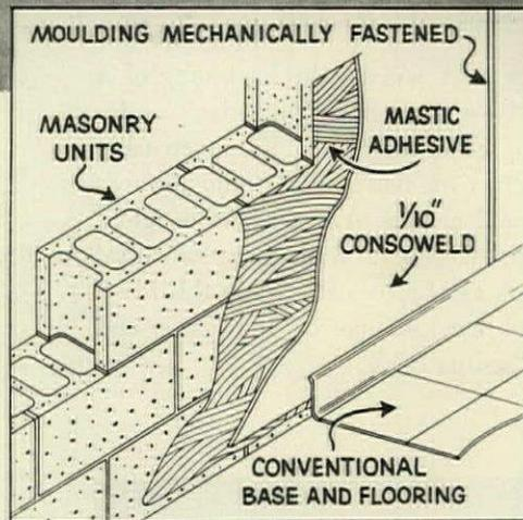
Consoweld 10 lends itself to all types of vertical surfaces. It can be applied directly over plywood, gypsum board, gypsum lath or masonry units. Consoweld 10 is nationally distributed by more than 100 distributors strategically located across the country.
