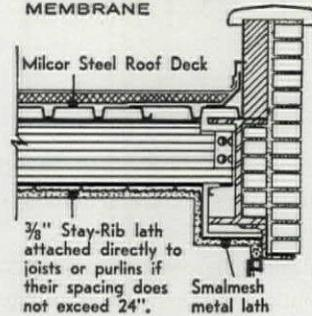
Membrane fireproofing protects beams, girders, and columns as effectively as concrete encasement, yet weighs considerably less.
