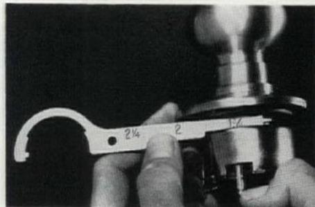
2 When spring-loaded pin is pulled back, rose rotates freely for easy adjustment. Combination spanner wrench and gauge provide exact positioning of rose.
