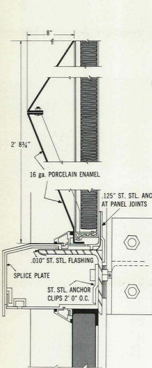
2. Vertical Section of Sill—Raised Porcelain Enamel Panel to Spandrel Panel.
