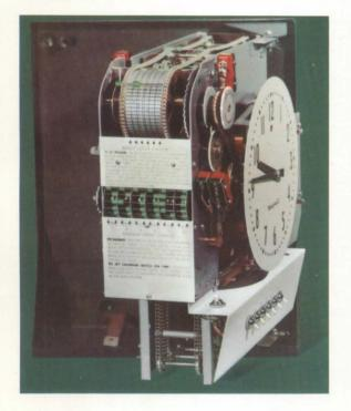
**Easy-to-set signal drum.** Honeywell's Clockmaster eliminates fuss and bother from program setting. Just turn signal drum to time, slip steel pin through chain links and slide on one of the reusable plastic rollers. To change signal, roller can be shifted without affecting any other part of the program. Special round pin-in-square-hole construction holds each signal roller firmly in place.
