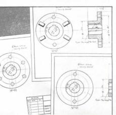
Make quick corrections over scattered areas. When small patches of your original drawing need alterations, make a Vapo-Vel intermediate. Then eliminate the unwanted lines with POST Eradicator Fluid and redraw.
