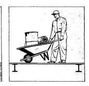
**STRENGTH.** Angular pattern with wide rib openings provides strong section properties. Granco Deck supports wheelbarrows, welding machines, etc., without bending or backting.
