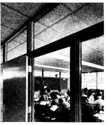
**CLASSROOMS** and corridors feature Tectum acoustical ceiling panels, one inch thick. Ceiling height partitions are possible with Tectum's high sound transmission loss. Tectum minimizes sound transmission over the partitions.
