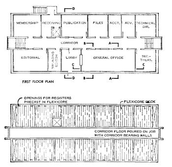
First Floor Framing. Corridor floor was cast in place with corridor bearing walls. Flexicore clear-spans from corridor walls to outside walls.
