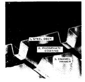
**TOUGH FINISH.** Rust-preventive enamel is "flow coated" over steel, baked on at 350° F. for 20 minutes. Flint-hard finish prevents corrosion, resists abrasion from field handling.
