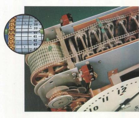
**Easy-to-read numbers: Link chain ruggedness.** Numbers on the signal drum are large, easy to read, and never confuse the program setter. Two precision link chains, color-coded for day-night identification, guide the entire program whether it includes three circuits or six. Chains are rated at twenty times load for insurance against breakage. Chains run continuously over idler gears. No piling at bottom of cabinet.
